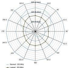
Note: All measurements reflect output power of 4W EIRP
